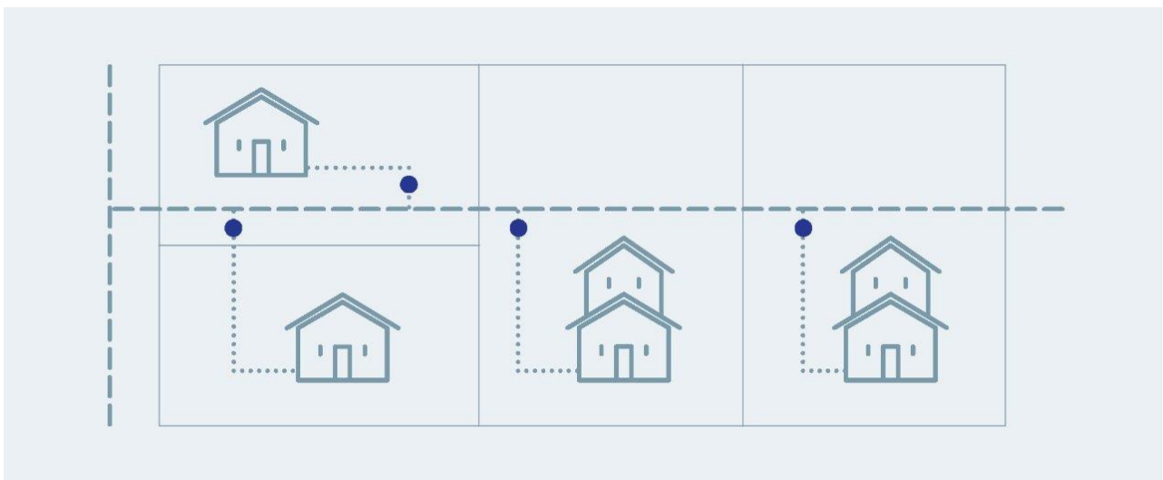
Figure B2 Council Wastewater Pipe through Private Land
