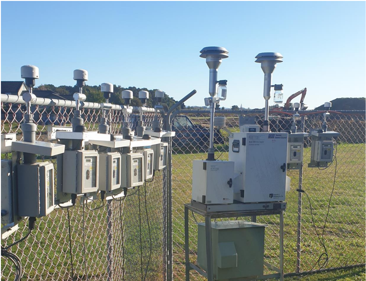
Figure 3: Photograph of the ES642 units co-located alongside the TDC Partisol in Brightwater.
