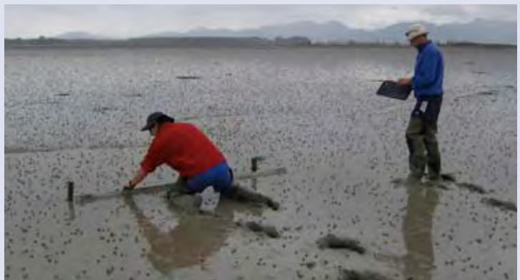
Measuring sedimentation rate in soft muds in Waimea Inlet.
