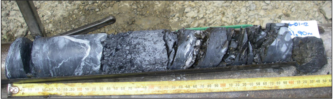
Figure 11: DH10 sheared zone at 31.6 m as recovered.
