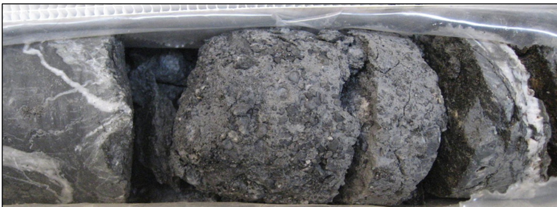
Figure 12: DH10 Shear zone with plastic clayey gouge and rock fragments at 31.6m
