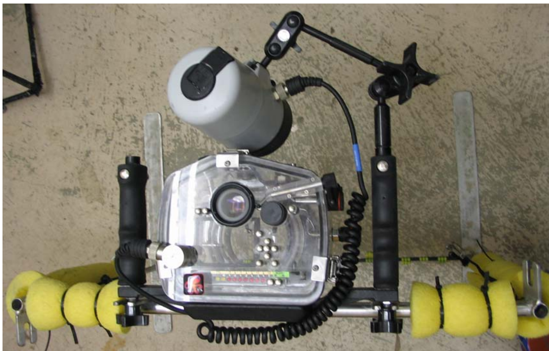
Figure 2. Quad cam apparatus for collecting seabed images.
