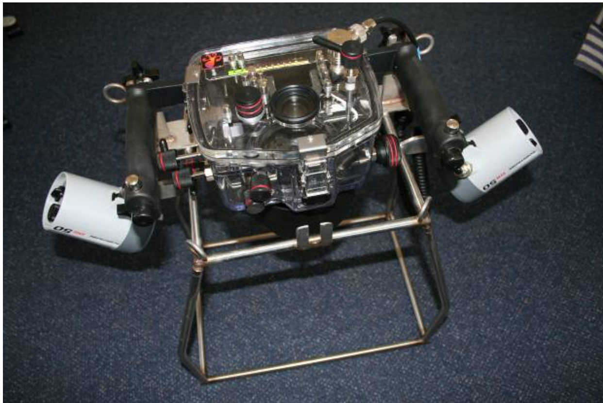
Figure 2. Quad cam apparatus for collecting seabed images.
