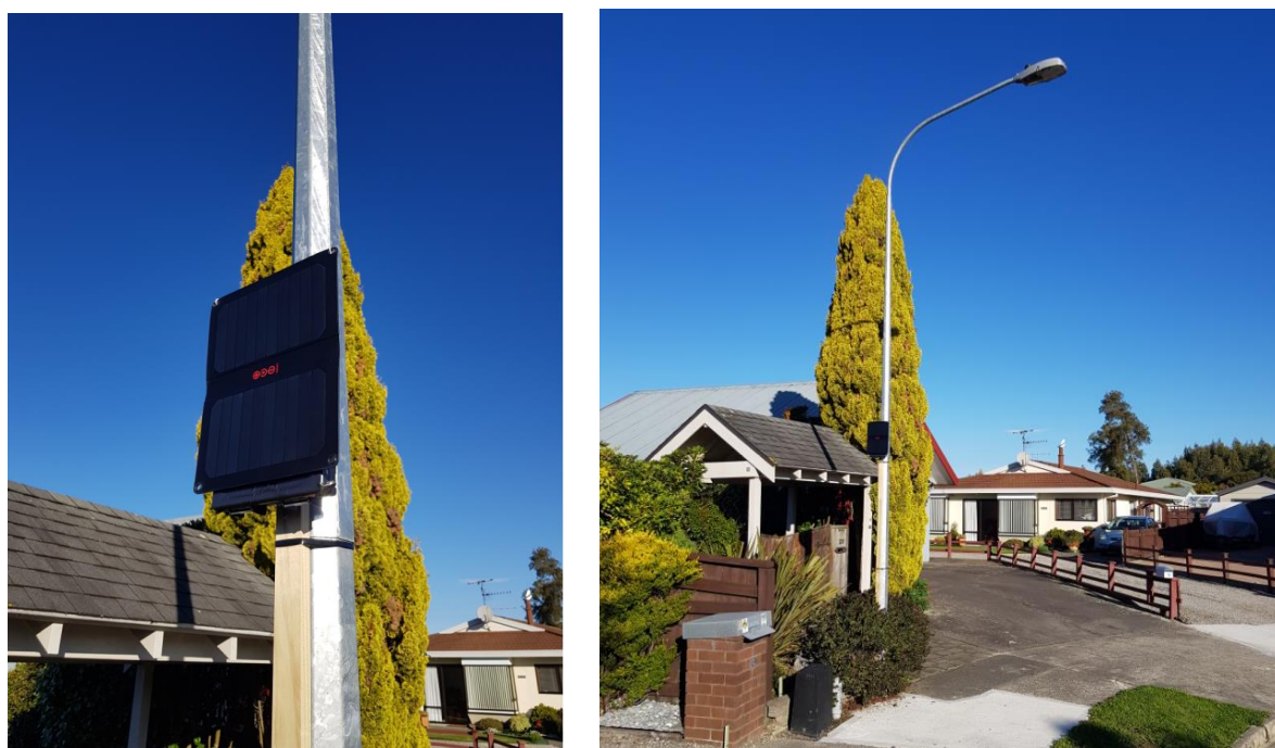
Figure 1: ODIN low cost sensor package in-situ.
