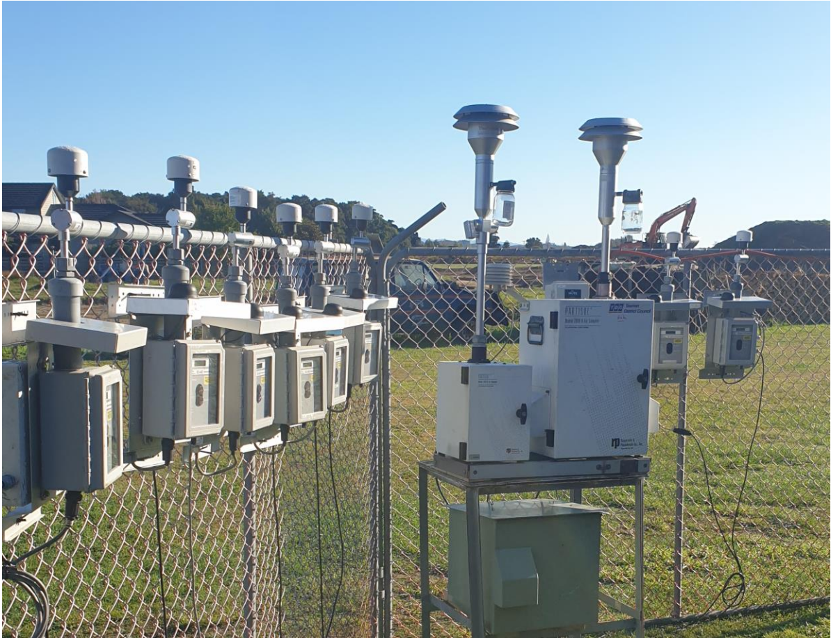
Figure 1: Photograph of the ES642 units co-located alongside the TDC Partisol in Brightwater.
