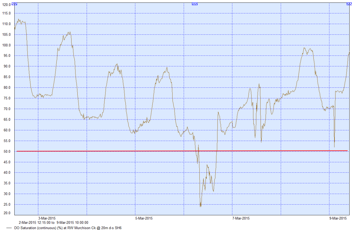
Figure 14. Dissolved oxygen % saturation at Murchison Creek 20 m downstream of SH6 from 2-9 March 2015. The national proposed bottom line for the daily 1-day minimum is shown by the red line.
