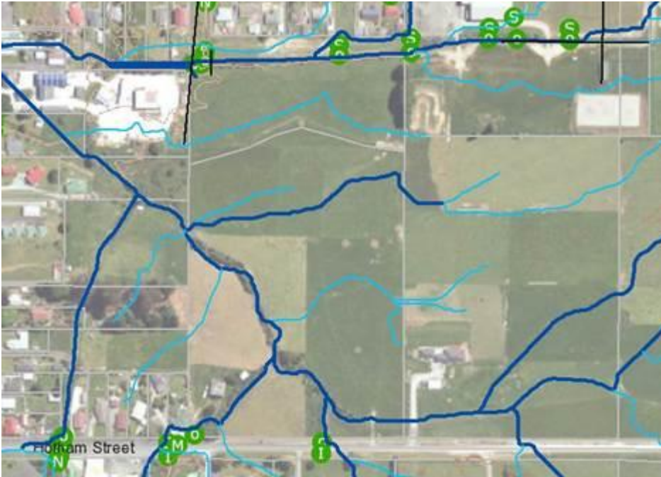
Figure 11: Estimated overland flow paths - 65 Hotham Street (Email from Emma McFarlane, Stormwater Planning Advisor, 10 December)
