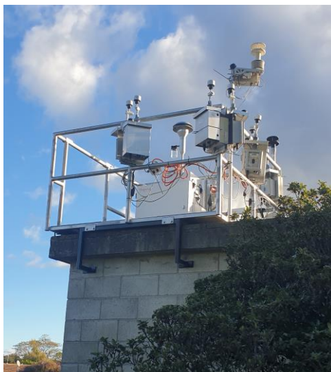
Figure 3: Photograph of the ES642 units co-located alongside the TDC Partisol at Goodman Ledger Park, Motueka.
