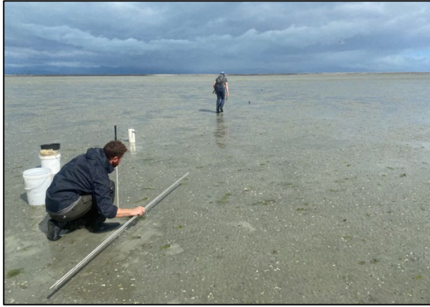
Example of measuring sediment plate depth. A straight edge is used to account for irregularities in the sediment surface. Depth is measured in triplicate to the nearest millimeter and recorded as an average per plate.
