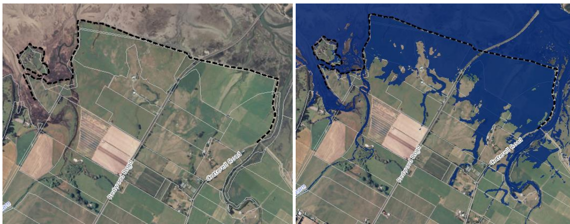
Figure 6: Farmland presently protected from tidal inundation during a MHWS tide (left image) but potentially affected by the tide (right image) in the absence of the tide bank
