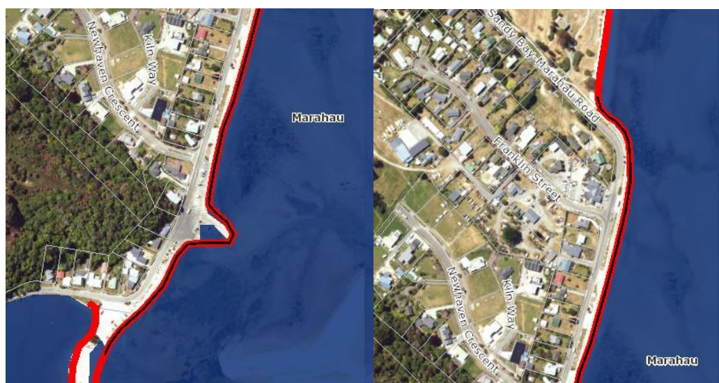
Figure 7: Coastal erosion (red line) and coastal protection structures (black line) at Marahau
