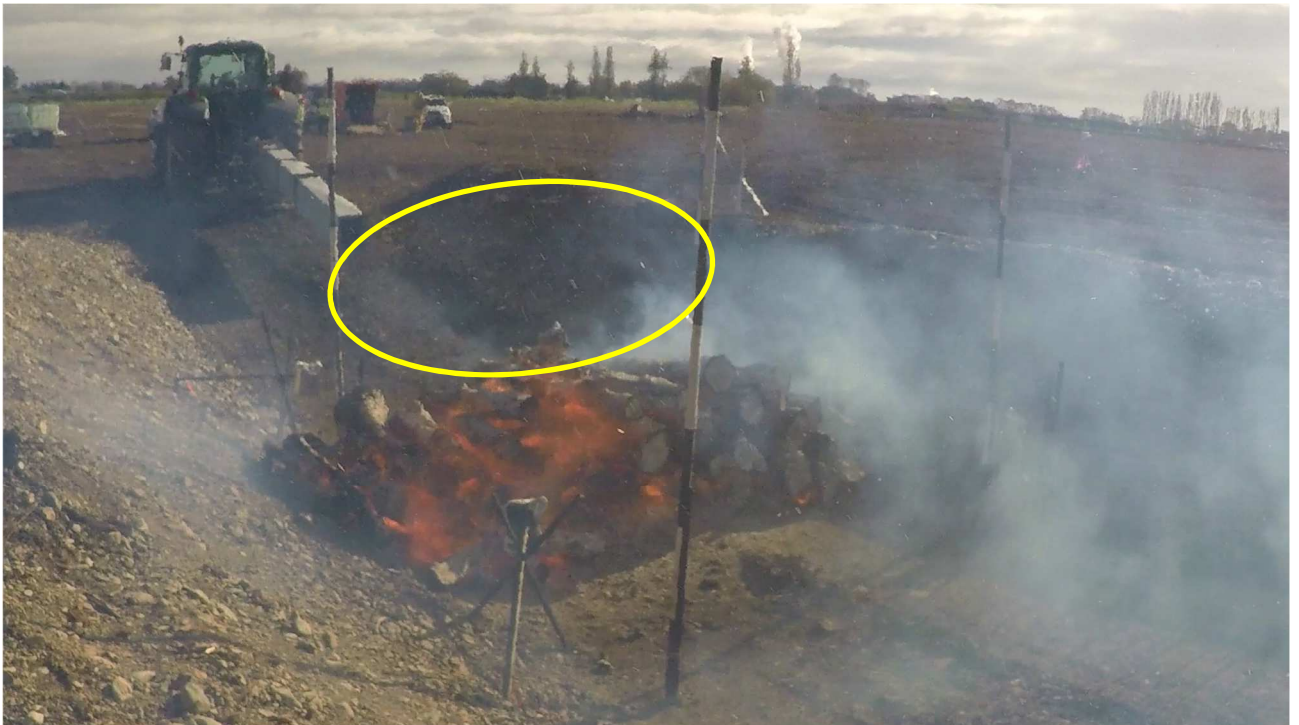
Figure 15: Soot particles (circled in yellow) lofted into the air by the fan used during Burn 3.
