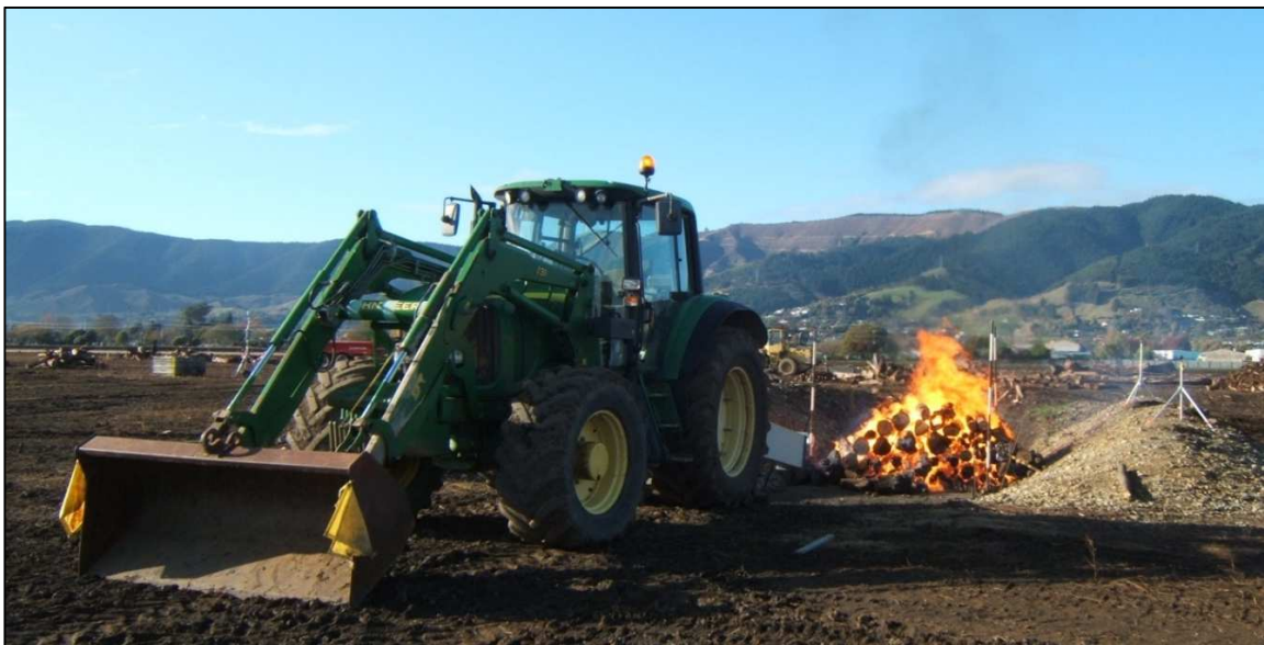
Figure 2: The setup for Burn 3 – New Technique. The burn pile was placed inside a trench and a fan, mounted on the back of a tractor, blew onto the fire. Note very little visual smoke emitted from the burn, indicating efficient combustion.
