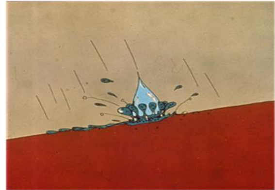
Figure 3-5 Schematic of Raindrop Splash
