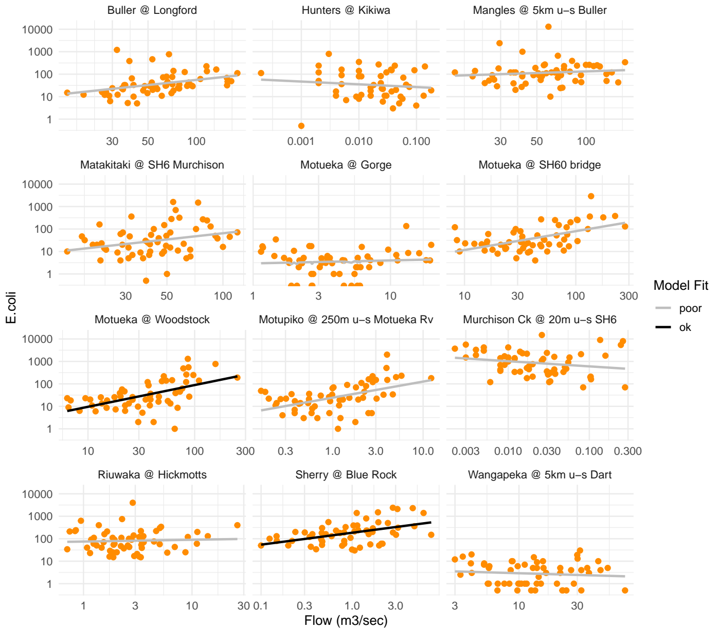
Figure 44: E. coli concentration (cfu/100ml, log10-transformed) and river flow (m3/sec) over 5 years with LogLog fitted line. Model fit = *poor* when less than 20 percent of the variation in E. coli was explained by flow.
