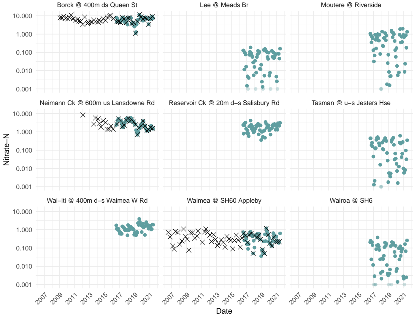
Figure 31: Nitrate-N data (g/m 3 , log 10 -transformed) sampled monthly over 5 years (dots) and quarterly over 15 years (crosses). Values below detection are lighter in colour.
