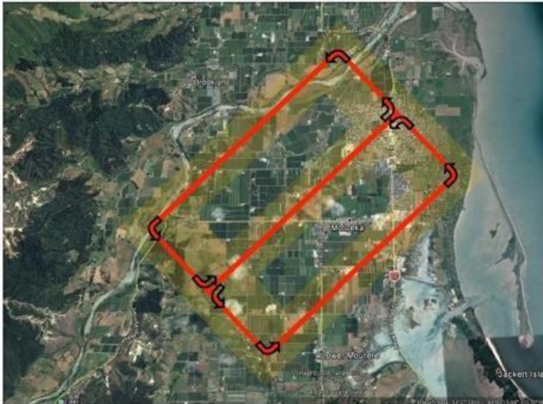
The circuit is an orderly pattern used to position the aeroplane for landing and minimise the risk of collision with other aircraft.
