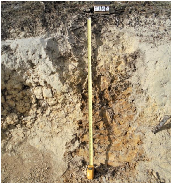
Figure 6. Mapua soil profile showing blocky structured subsoil and typical bleaching of the soil surface on an exposed cutting.
