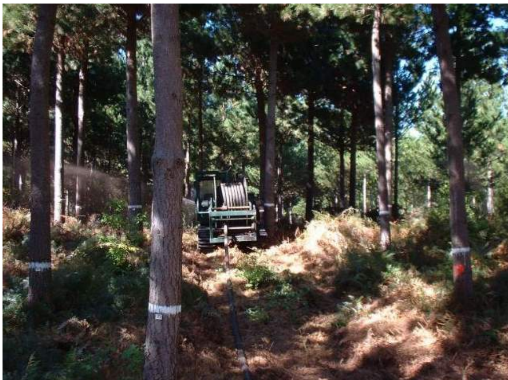
Figure 4: Travelling irrigator for biosolids application within a stand of trees on Moturoa/Rabbit Island
