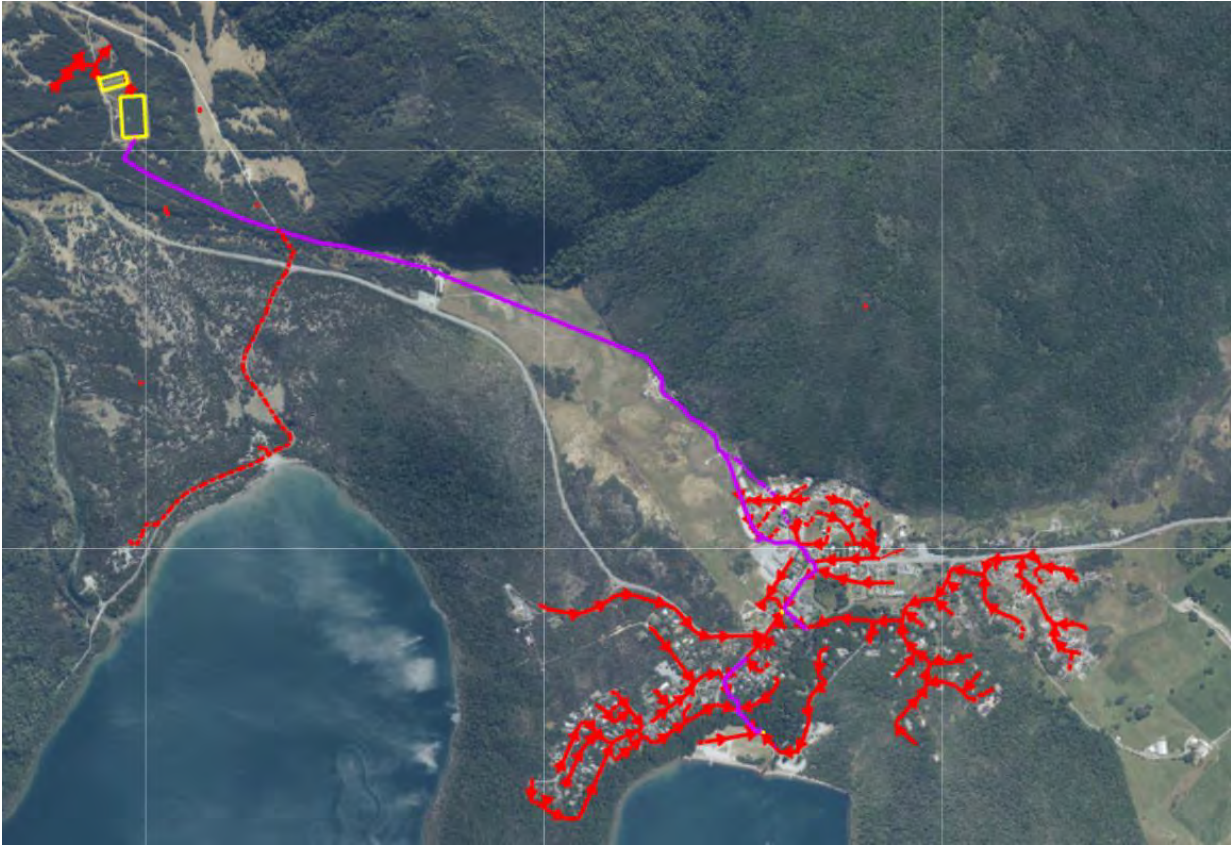
Figure 4 St Arnaud wastewater network
