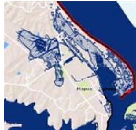
2. Current high tide mark (solid dark blue) and 1% annual exceedance probability for salt-water intrusion (hatched dark blue)
