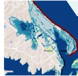
3. Salt-water intrusion under 0.5M sea-level rise, mean high tide mark (solide blue) and 1% annual exceedance probability (hatched blue)
